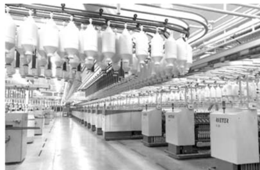
Perfect, contact-free bobbin transport ensures consistent quality
